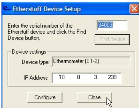
If your LAN supports DHCP, your ET-2RHT will have a meaningful IP address already in the IP address field of Etherset; write it down and click close. If your LAN doesn't support DHCP or you wish to assign a Static IP to your ethermometer, enter the static IP in the IP address field and click configure, then close. You can also change to a static IP or change the one assigned here at any time from the unit's web interface.
